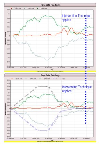
The underlying algorithm that "pattern matches" to arrive at a probability of the data being root induced clay shrinkage has been superimposed on the lower image - there is a greater that 85% probability that movement here is root induced.
