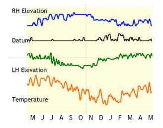
The black line is the datum, fixed to the LH side wall of the house. It is also being influenced by tree root activity, although less than the electrolevels fixed to the LH side wall of the extension, nearer to the trees.
