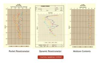
Above we reproduce the results from tests undertaken at the BRE research site at Chattenden. The characteristic bulge of root induced clay shrinkage is clearly visible. The rig penetrometer matches the profile obtained using the neutron probe at Aldenham. At shallow depth we see the influence of ground evaporation, and at around 2mtrs bGL is the root induced bulge, each diminishing with distance from the row of Poplars.
