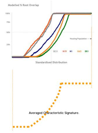
Above is the 'percentage overlap' estimate based on the statistical assessment of root zones encroaching beneath a building derived from claims data.
